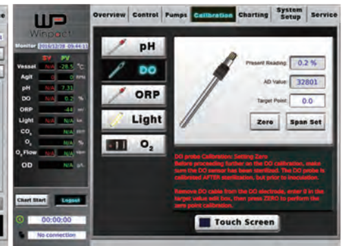
Calibration Easy sensor calibration with assisted menu
