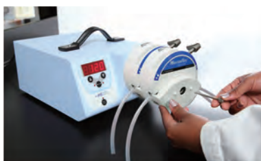
Easy load pump head with reversible flow for purging purposes
