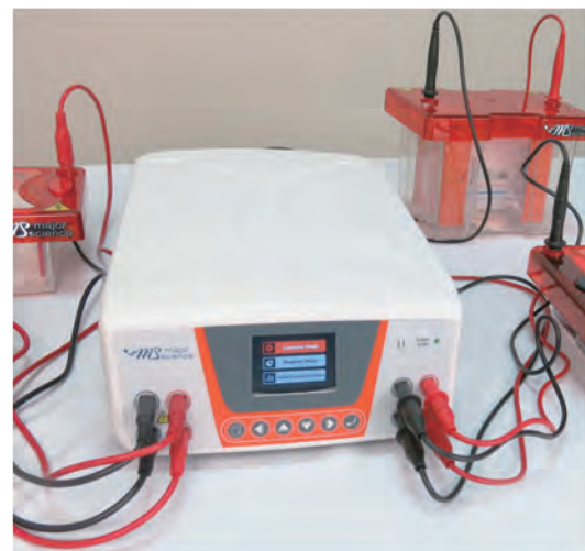
Four pairs of outlet terminals
