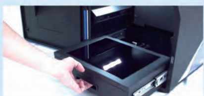
Pull out UV transilluminator
