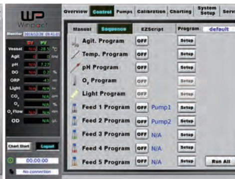
Control / Manual Manual operation, sequence or EZScript control (optional) of each parameter.
