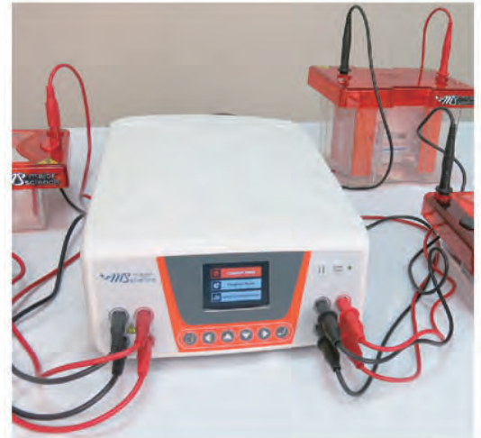
Four pairs of outlet terminals
