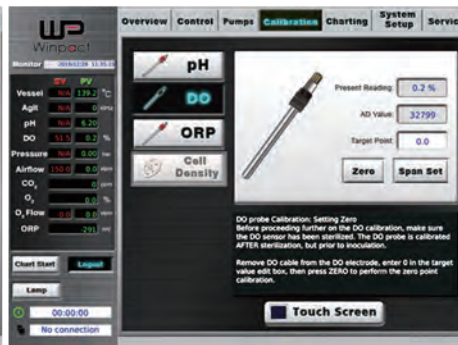
Online system calibration with system feedback
