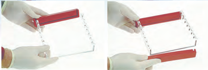
Casting dams allow gels to be rapidly cast
