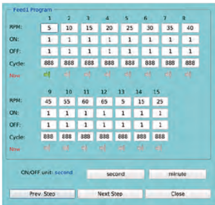
15-Step programmable PID control
