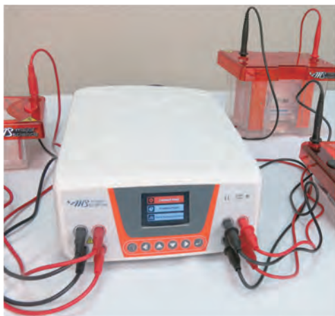
Four pairs of outlet terminals
