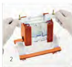
2 Transfer to casting base and tighten cams.
