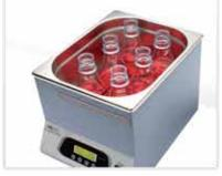
Max. chamber capability (no using stirring mixture function): 6 sets of 250ml flasks 4 sets of 500ml flasks
